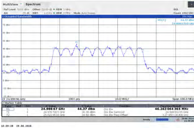
n258-b 50MHz-16QAM-Mid CH-32RB0
