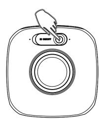
To turn ON the speaker, press and hold the Multifunction Button for approximately 2-3 seconds. The indicator light will flash blue as it enters pairing mode.
