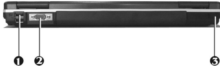
1. USB 2.0 Ports 2. VGA Port 3. Kensington Lock Hole
