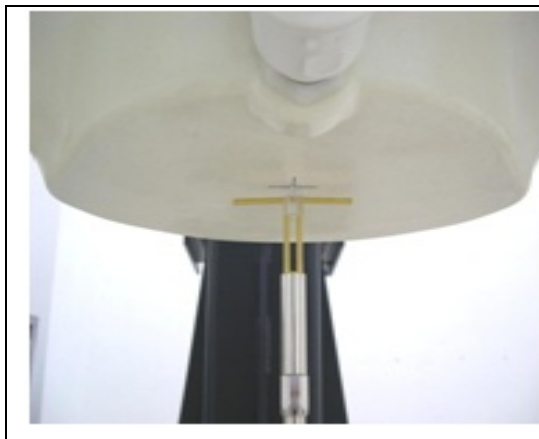
Fig 7.1 Photo of Dipole Setup
