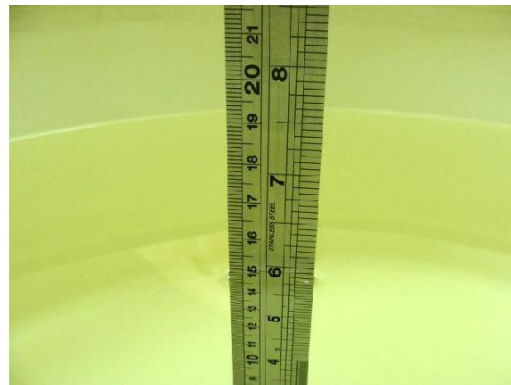
Fig 6.11 Photo of Liquid Height for Body SAR
