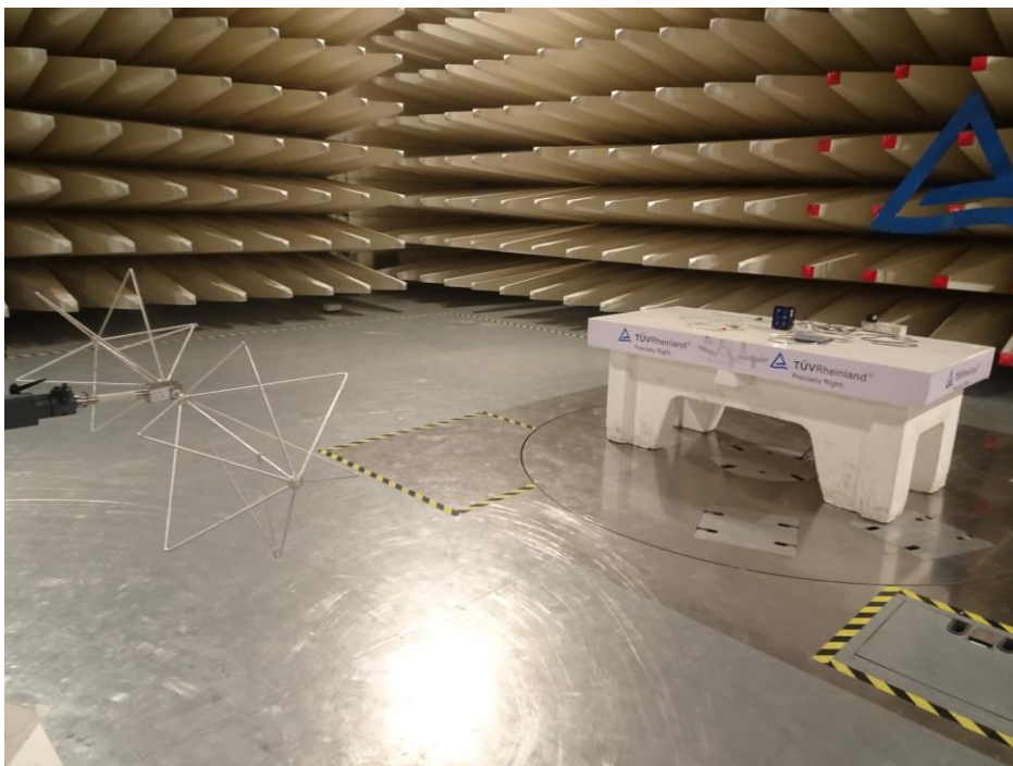
Test setup Frequency Range 30MHz-200MHz Biconical Antenna
