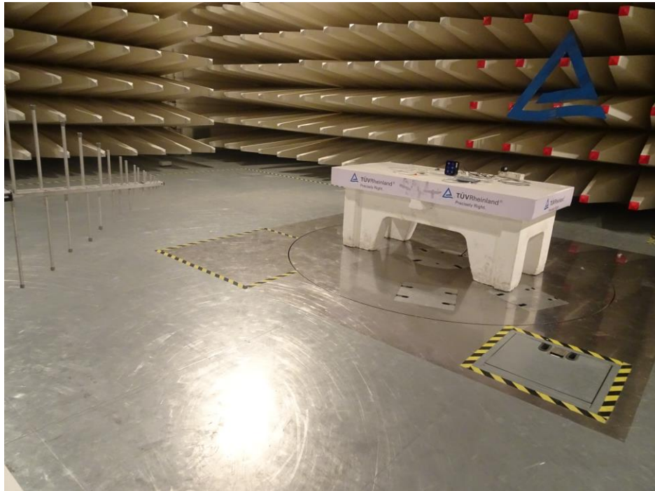
Test setup Frequency Range 200MHz-1GHz Log periodic Antenna
