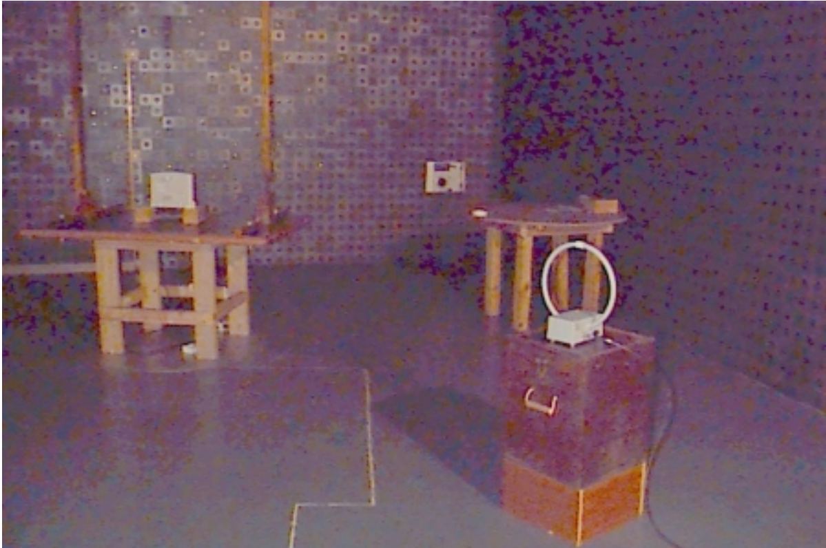
Photograph No. 4.8.1 Radiated emission measurement test setup
