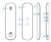
. 2. Indication LED 7. Power on Off Key 3. Button A 8. Volume + 4. Button B 5. Microphone
