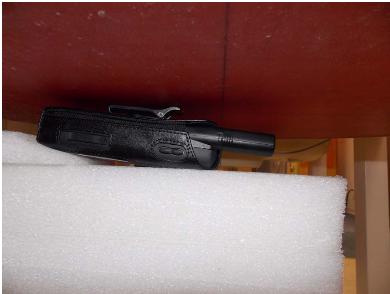
Test Position Body Retracted Touch 0 mm Gap
