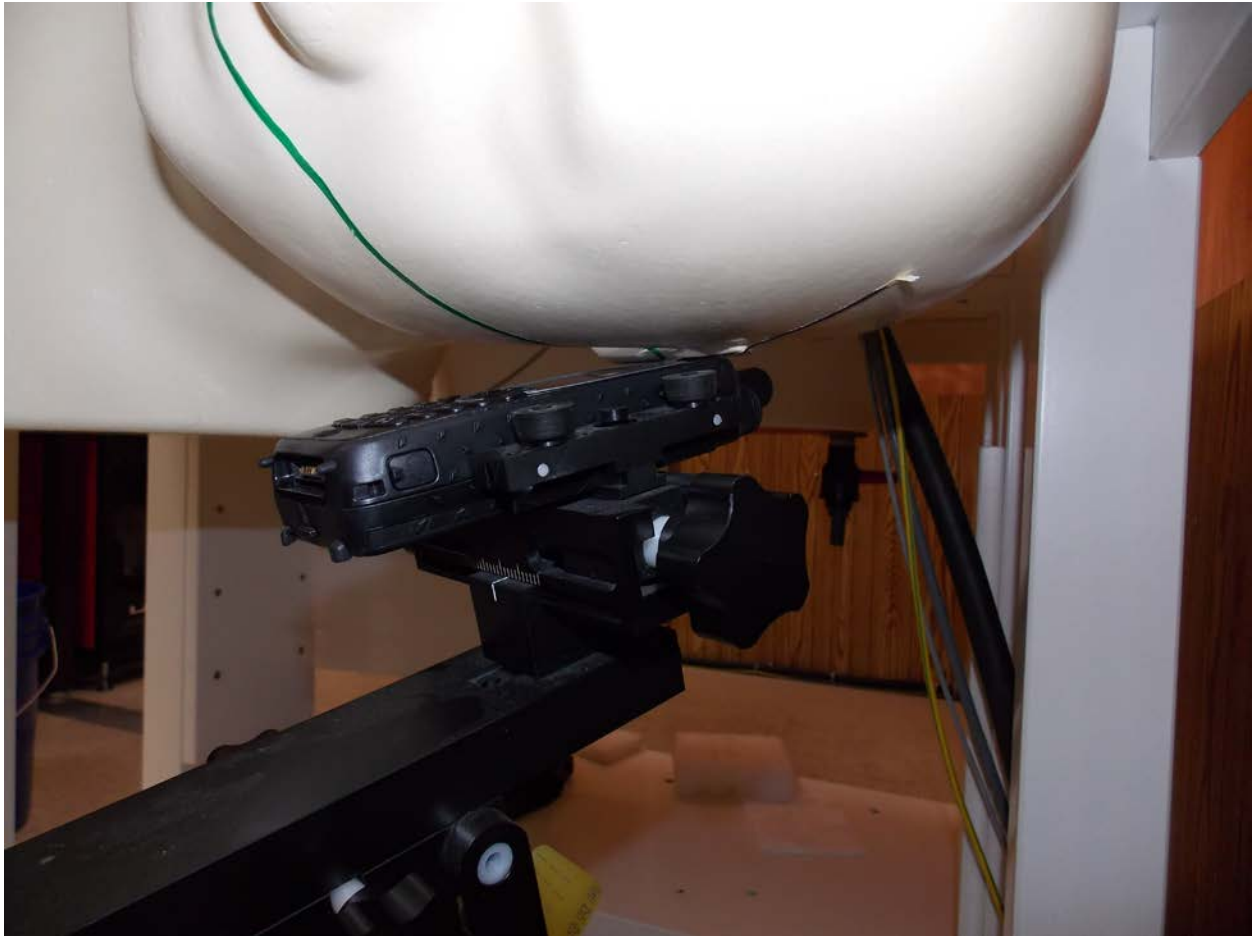
Test Position Left Head Retracted Tilt 0 mm Gap
