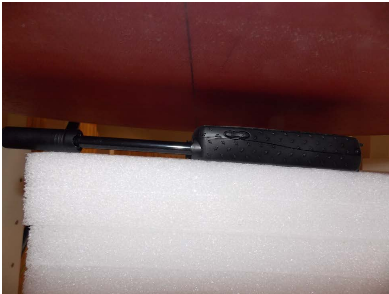
Test Position PTT Face Extended 25 mm Gap
