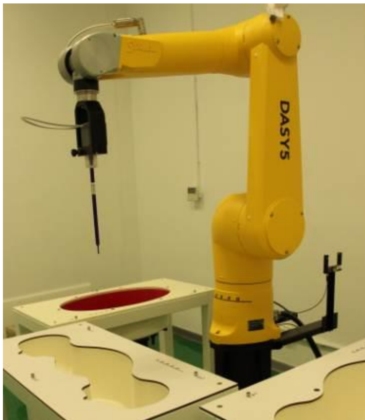
Picture 8-7: Specific Absorption Rate Test Layout
