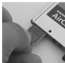
Figure 2-1: Inserting the SIM card into the AirCard SIM card slot
