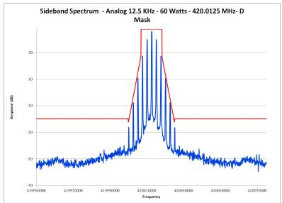
E1-5.29 Occupied Bandwidth, Analog, 12.5 kHz Channels, 420.0125 MHz PL
