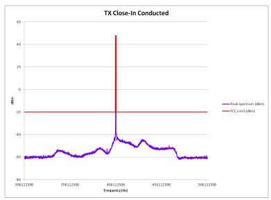
E1-6.4 Conducted Spurious Emission Spectrum, 200 MHz Span, Power 60 Watts, 420.0125 MHz
