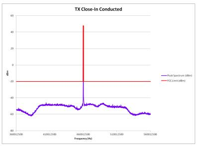
E1-6.8 Conducted Spurious Emission Spectrum, 200 MHz Span, Power 60 Watts, 469.9875 MHz
