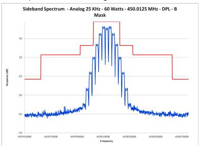
E1-5.19 Occupied Bandwidth, Analog, 25 kHz Channels, 460.0125 MHz
