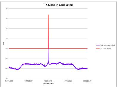
E1-6.7 Conducted Spurious Emission Spectrum, 200 MHz Span, Power 60 Watts, 460.0125 MHz
