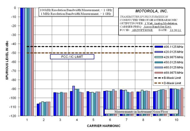
E1-6.3 Conducted Spurious Emission Spectrum, 200 MHz Span, Power 60 Watts, 406.1125 MHz
