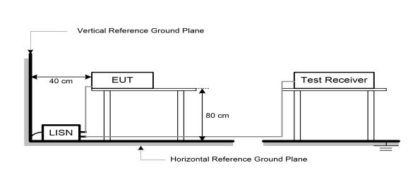
The LISN edge is arranged parallel to the edge of the test table The vertical conducting plane or wall of an RF-shielded (screened) room shall be located 40 cm to the rear of the EUT
