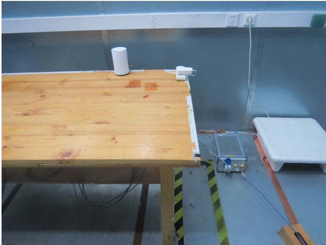
Picture 3 Conducted Emission Test Setup
