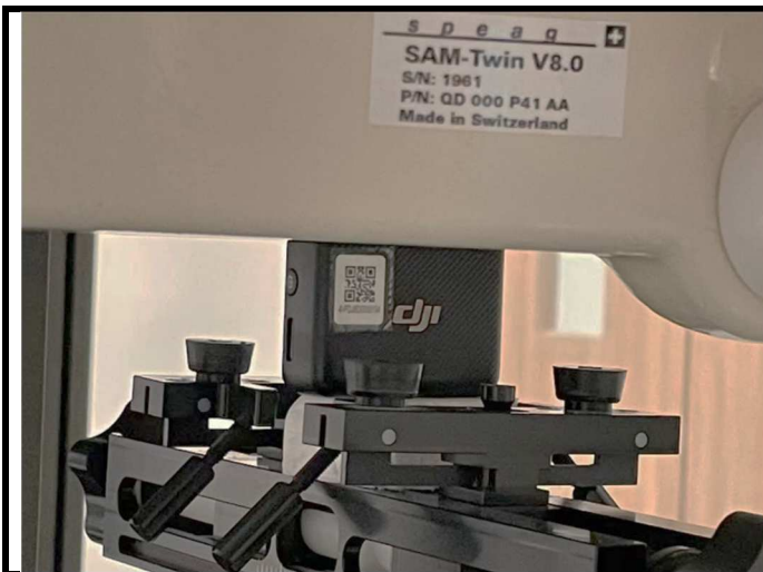
Front Face of EUT with 0 cm Gap
