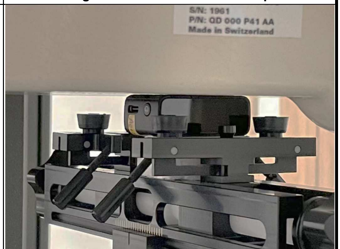
Bottom of EUT with 0 cm Gap
