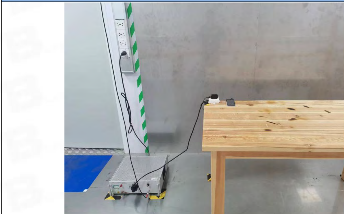
Conducted Emission at AC power line
