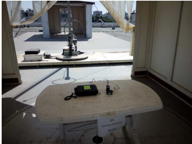
Figure 2. Radiated Emission Test
