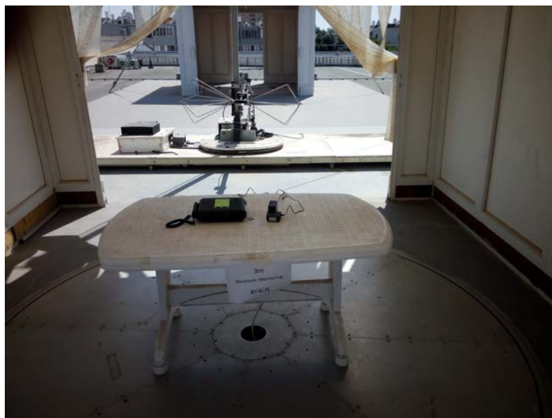
Figure 3. Radiated Emission Test
