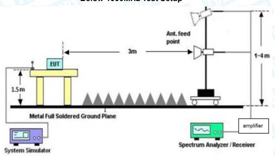
**Above 1GHz Test Setup**
