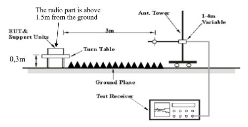
The radiated emissions were performed in the 3 meters distance, using the setup accordance with the ANSI C63.10-2013. The specification used was the FCC 15.209, and FCC 15.247,RSS-247,RSS-Gen limits.
