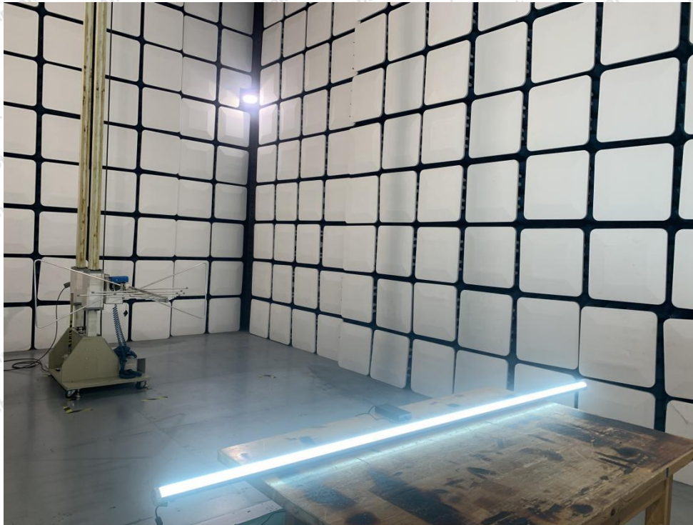
Photo of Radiation Emission Test
