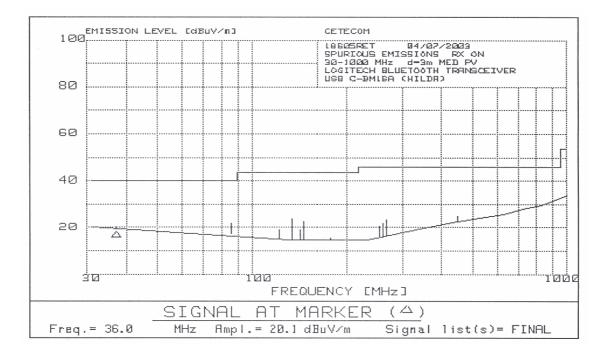
Resolution bandwidth= 100 kHz Video bandwidth= 100 kHz
