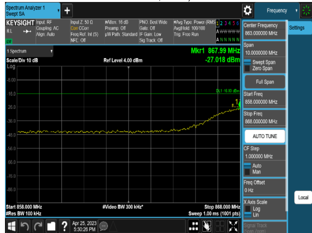
Plot 8-546. Conducted Spurious Emission Plot 858 MHz to 868 MHz (MSR 2C_DSS B(n)5_1C_10M+NR n5_1C_15M_2T_16QAM-Low Channel, Port 0)
