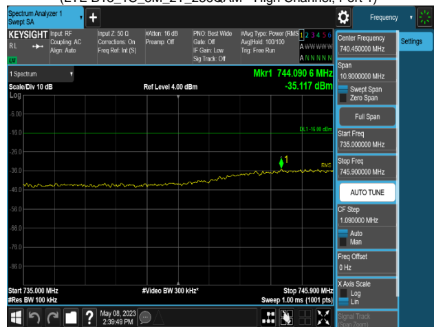
Plot 8-576. Conducted Spurious Emission Plot 735 MHz to 745.9 MHz
