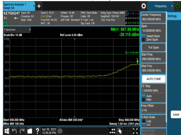
Plot 8-552. Conducted Spurious Emission Plot 858 MHz to 868 MHz (MSR 2NC_DSS B(n)5_1C_10M+NR n5_1C_5M_2T_QPSK-Middle Channel, Port 0)
