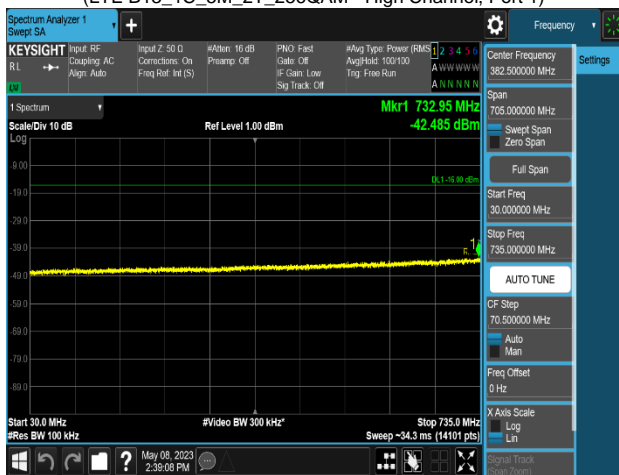
Plot 8-575. Conducted Spurious Emission Plot 30 MHz to 735 MHz
