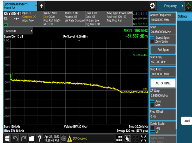
Plot 8-544. Conducted Spurious Emission Plot 150 kHz to 30 MHz (MSR 2C_DSS B(n)5_1C_10M+NR n5_1C_15M_2T_16QAM-Low Channel, Port 0)
