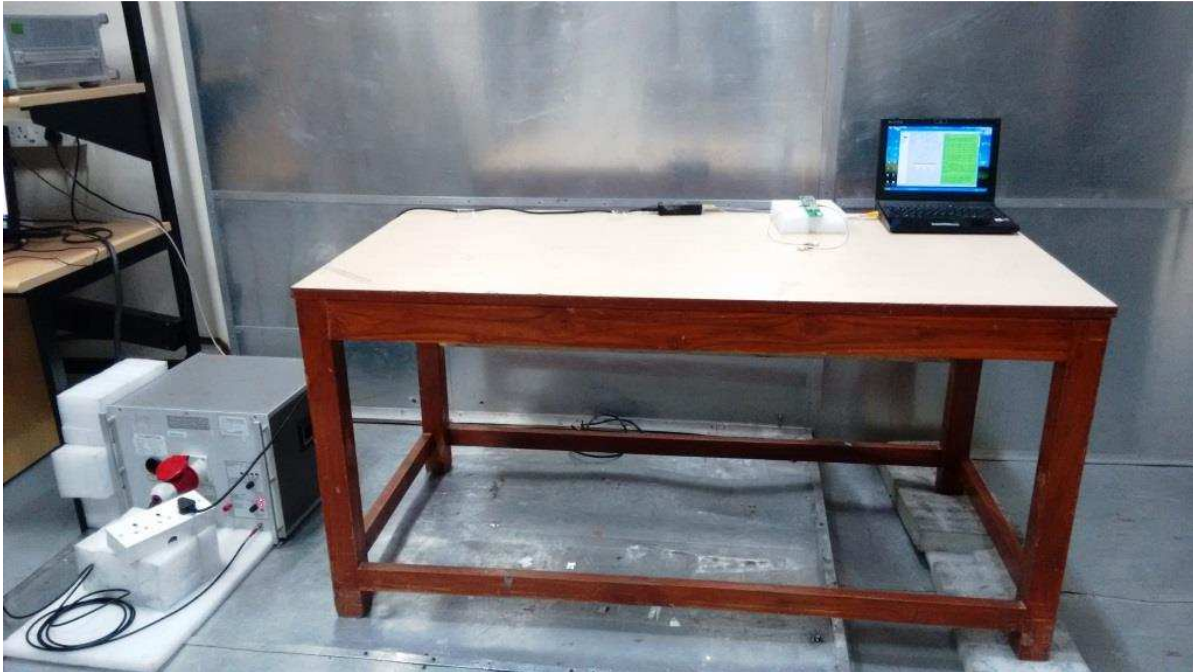
Figure 13: Conducted Emission Test set up photograph – 150 kHz to 30 MHz
