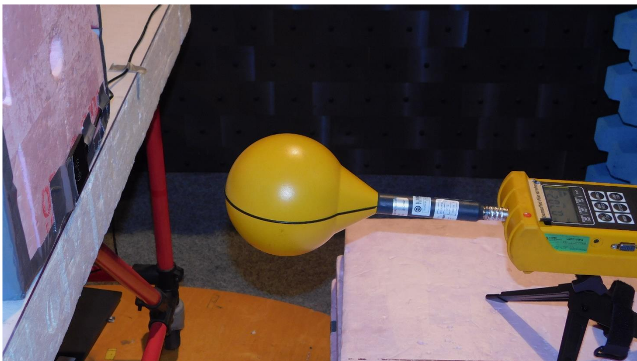
Picture 1: Setup of magnetic field test at a measurement distance of 20 cm, without RFID tag
