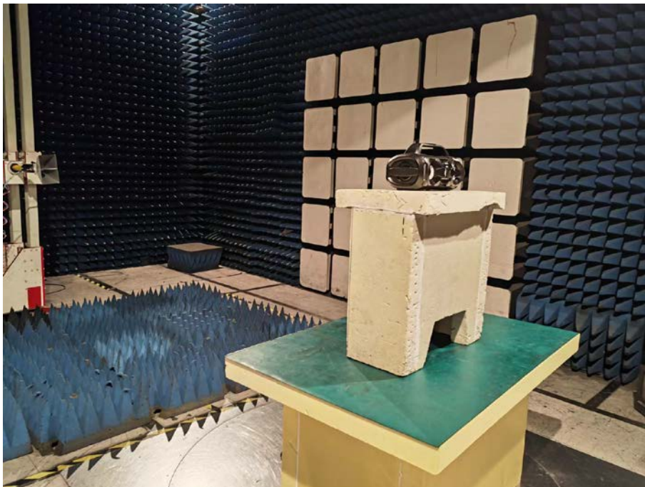
Spurious Emission Test Setup (Above 1GHz)
