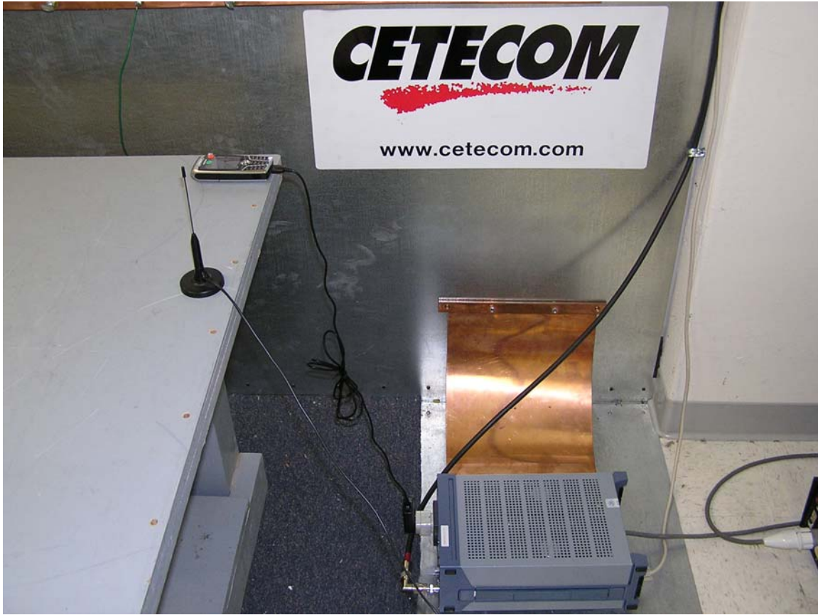
Test setup – AC Line Conducted Emissions
