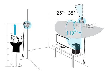
If your space doesn't allow for this kind of setup, you can also mount the base stations on tripods and light stands, or place them on stable surfaces such as a table.
