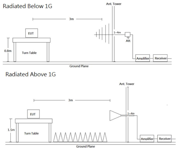
Radiated emission tests were performed in the 3 meters chamber test site, using the setup accordance with the ANSI C63.10-2013. The specification used was the FCC Part 15.209 and FCC 15.407 Limits.
