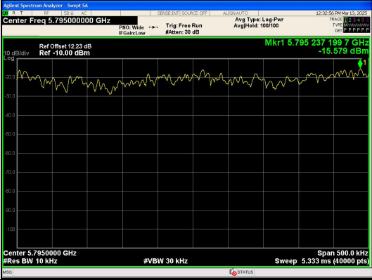
NT/NV_Antenna 0 IEEE 802.11n Channel 159 40MHz
