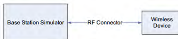
Figure 9.1 Power Measurement Setup
