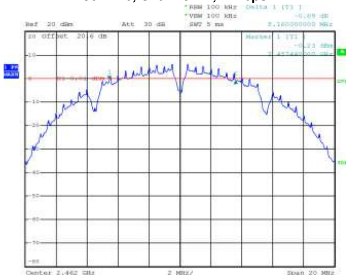
Figure 6-3: 6 dB Bandwidth 802.11b, Channel 11, 1 Mbps
