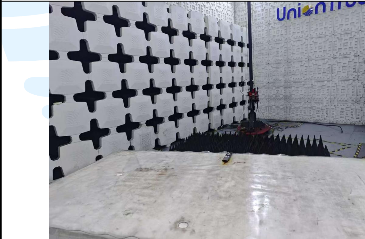
Radiated emission Test Setup-2 (Above 1 GHz)
