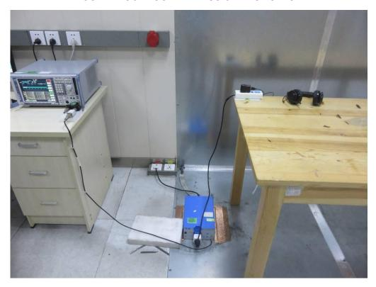
FCC RADIATED EMISSION TEST SETUP
