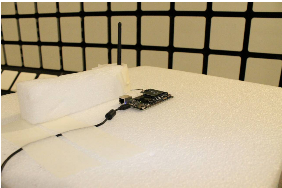
Photograph 4. EUT on table, BGM121N > 1GHz
