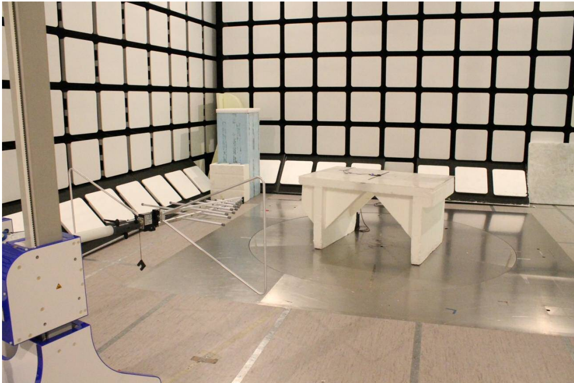
Photograph 1. Radiated Spurious Emissions 30 – 1000 MHz
