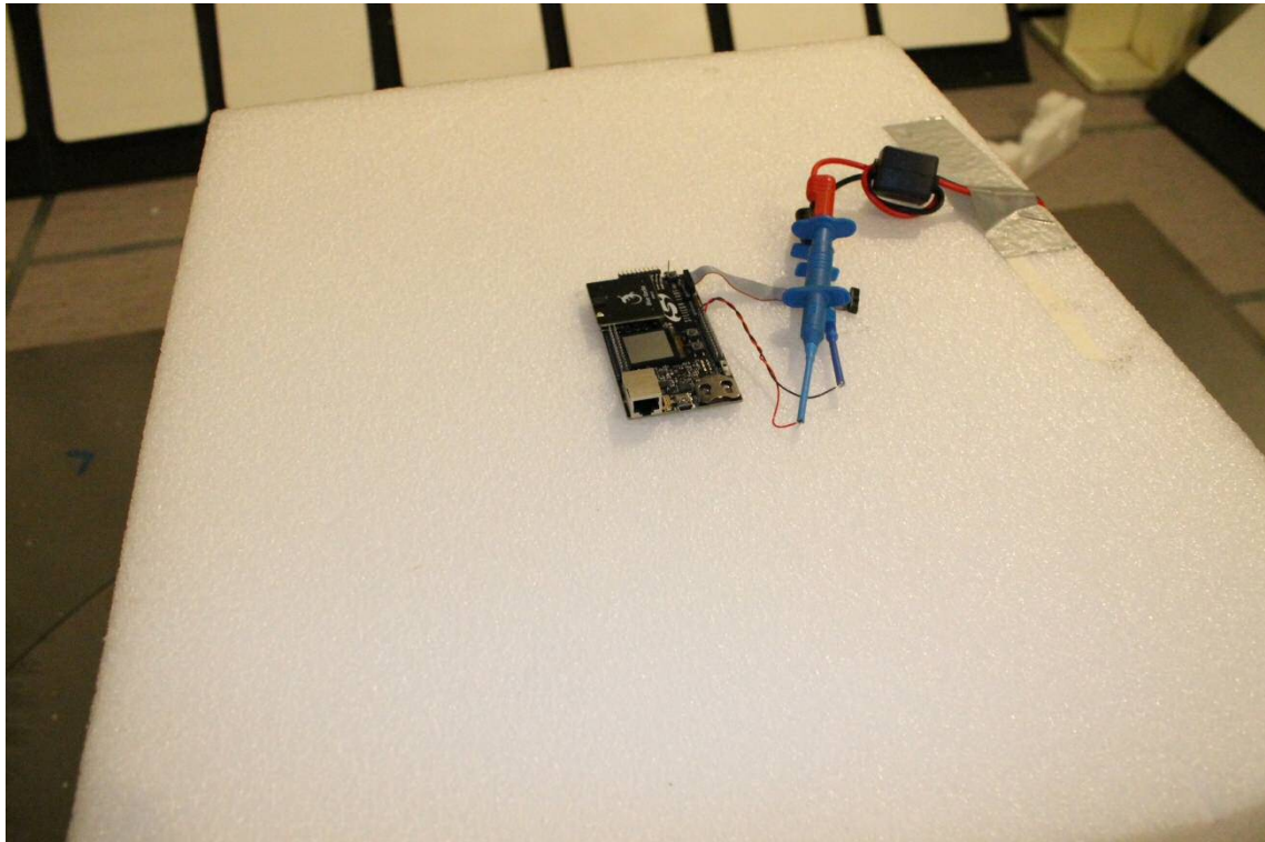
Photograph 5. EUT on table, BGM121A > 1GHz
