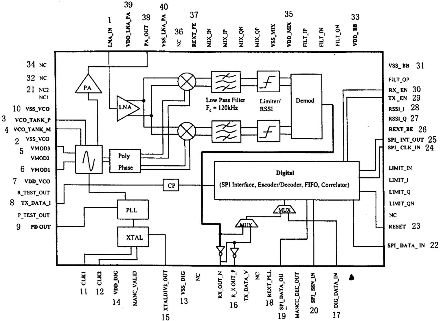
The ASIC main sections are a digital data interface, frequency synthesizer, transmitter (Tx) and receiver (Rx). The digital and frequency synthesizers both interface the Tx and Rx. To complete the transceiver function, several off chip components are required. The off chip components include:
