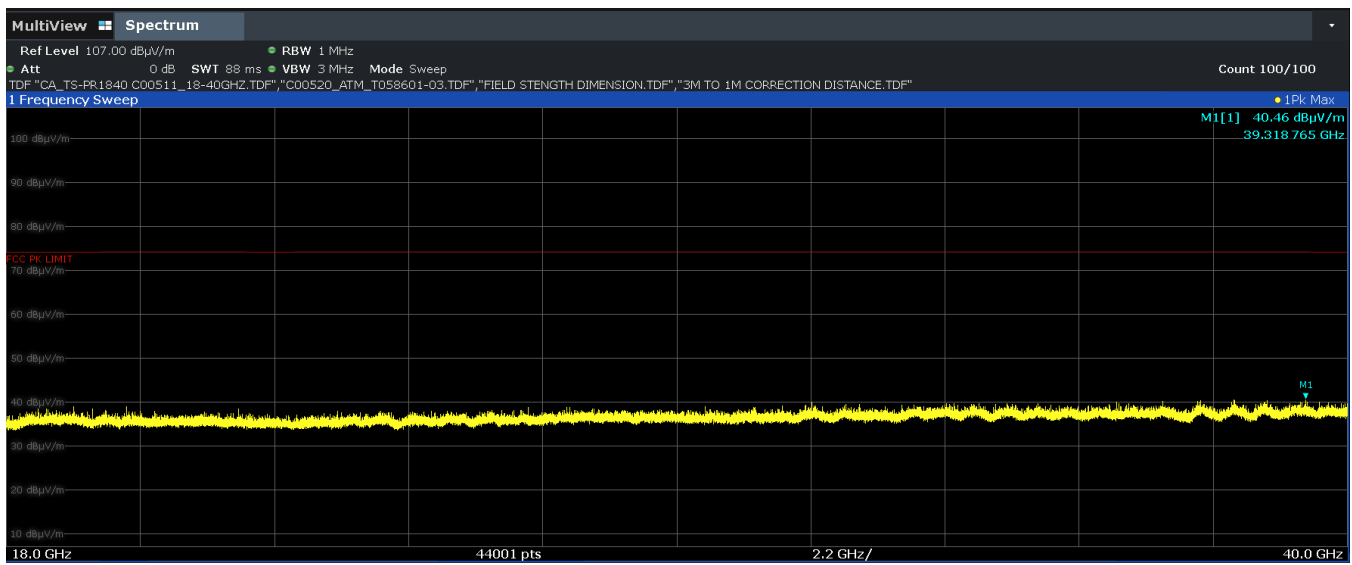
Plot 7-649. RSE 18GHz – 40 GHz CDD Primary (11ax Ch.116 — RU26, Pol. H)
