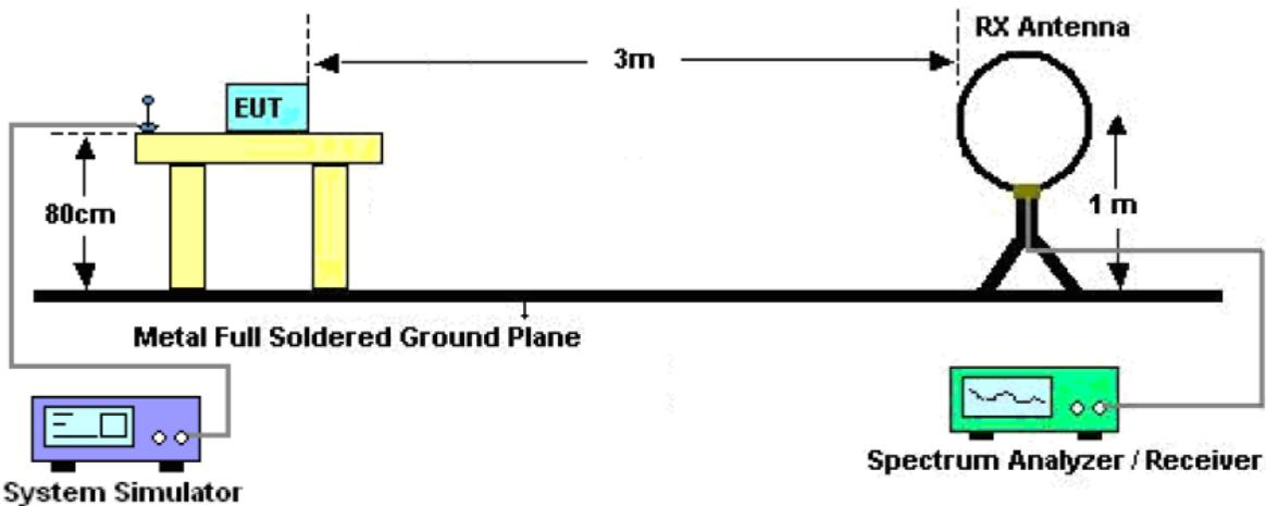
For radiated emissions from 30MHz to 1GHz
