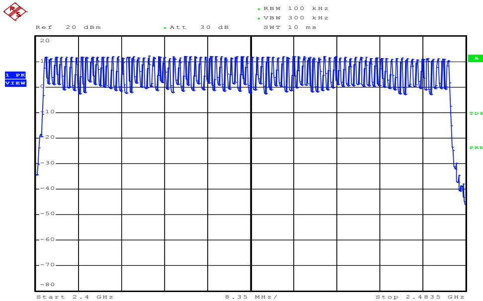
Modulation Standard:  $\pi/4$ -DQPSK (2Mbps)
