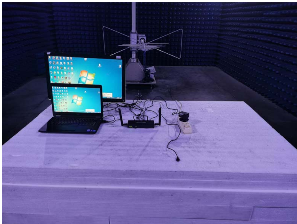
Photo of Radiated Emission Measurement (Below 1G)
