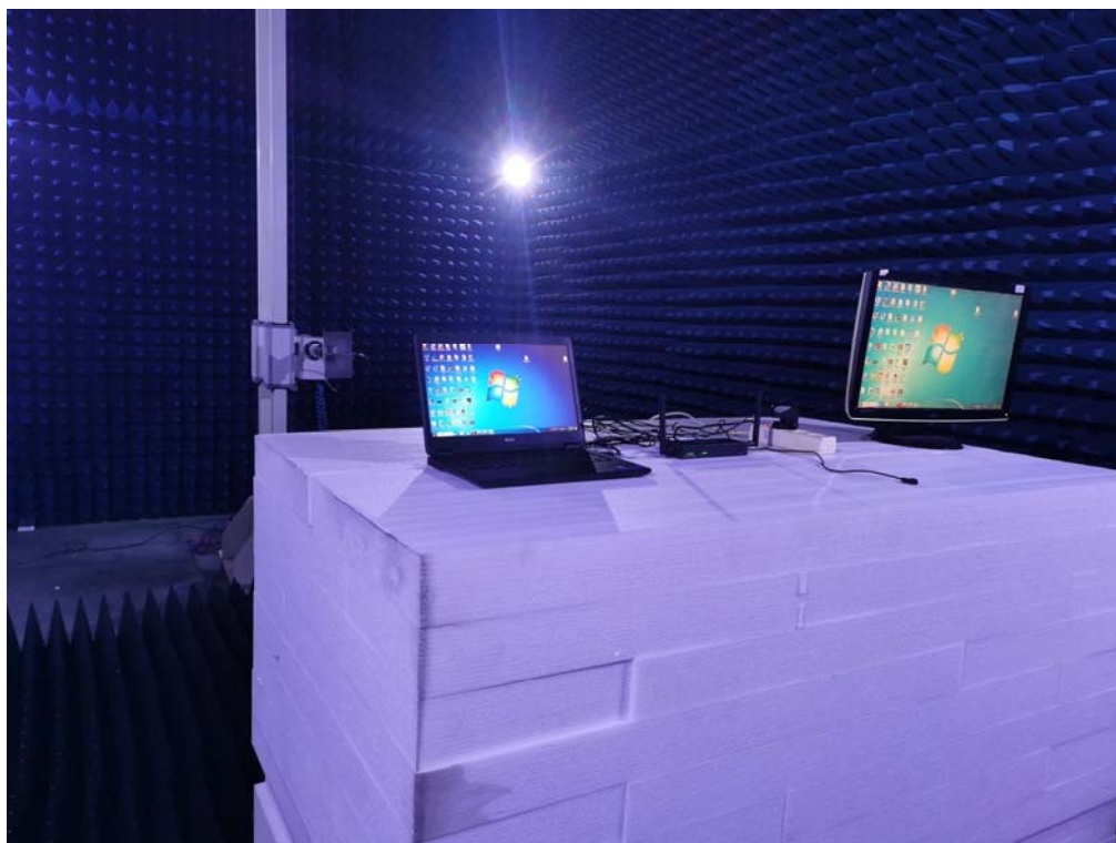
Photo of Radiated Emission Measurement (Above 1G)
