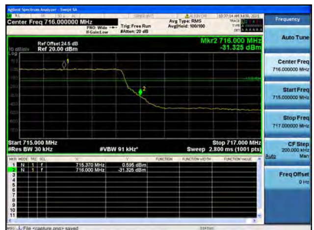
Band12 / 3MHz / High CH / QPSK / FULL RB
