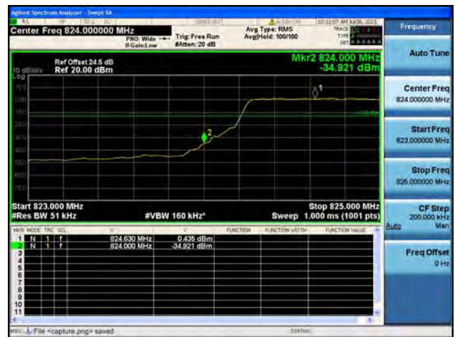
Band5 / 5MHz / High CH / QPSK / FULL RB
