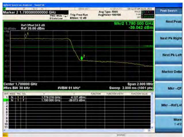
Band66 / 1.4MHz / High CH / QPSK / FULL RB
