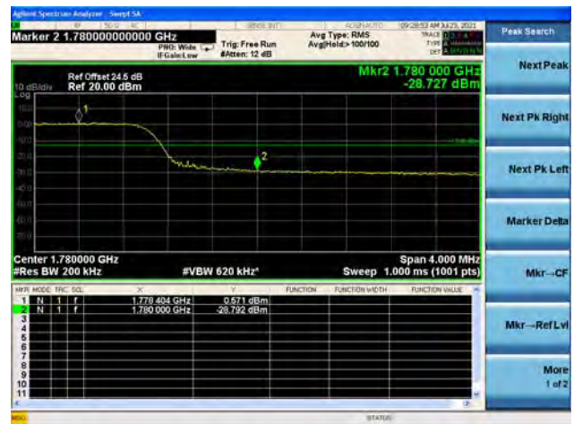
Band66 / 20MHz / High CH / QPSK / FULL RB
