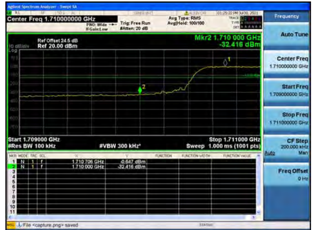
Band4 / 10MHz / High CH / QPSK / FULL RB
