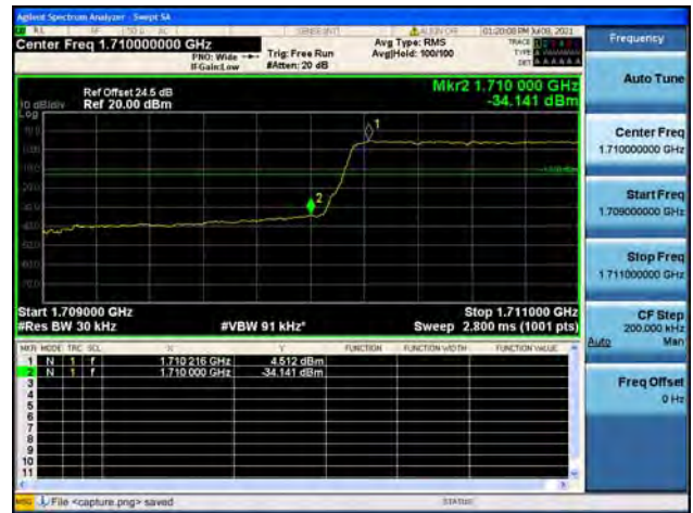
Band4 / 1.4MHz / High CH / QPSK / FULL RB
