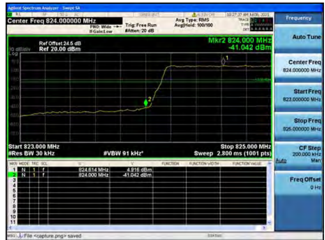
Band5 / 1.4MHz / High CH / QPSK / FULL RB
