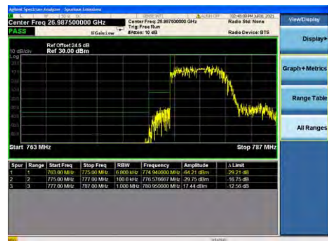
Band13 / 5MHz / High CH / QPSK / FULL RB
