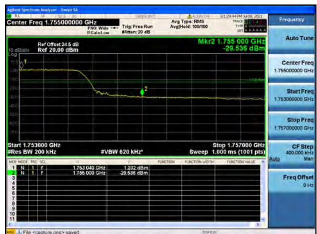
Band4 / 20MHz / High CH / QPSK / FULL RB
