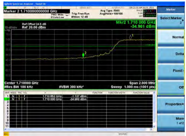
Band66 / 10MHz / High CH / QPSK / FULL RB
