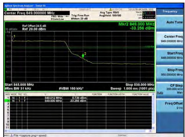
Band5 / 5MHz / High CH / QPSK / FULL RB
