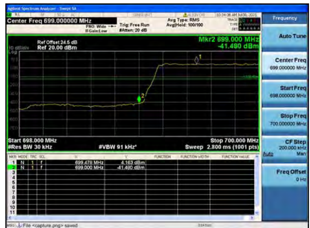
Band12 / 1.4MHz / Low CH / QPSK / FULL RB
