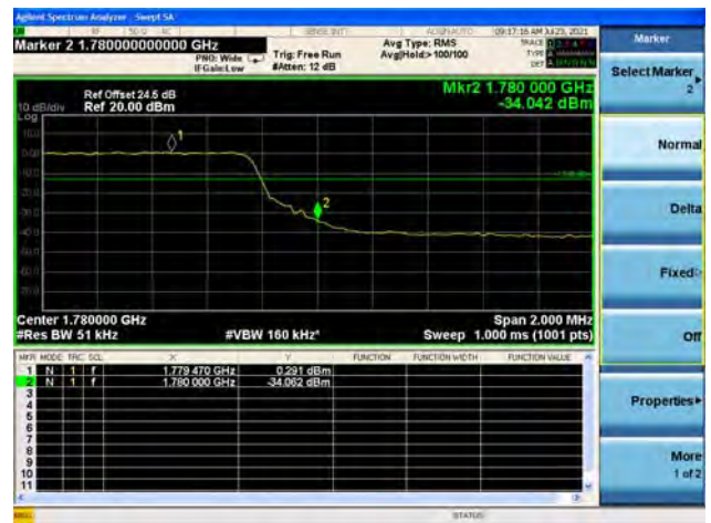
Band66 / 5MHz / High CH / QPSK / FULL RB
