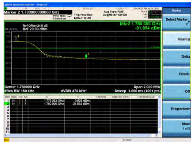
Band66 / 15MHz / High CH / QPSK / FULL RB
