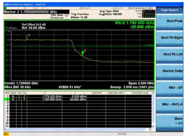
Band66 / 3MHz / High CH / QPSK / FULL RB
