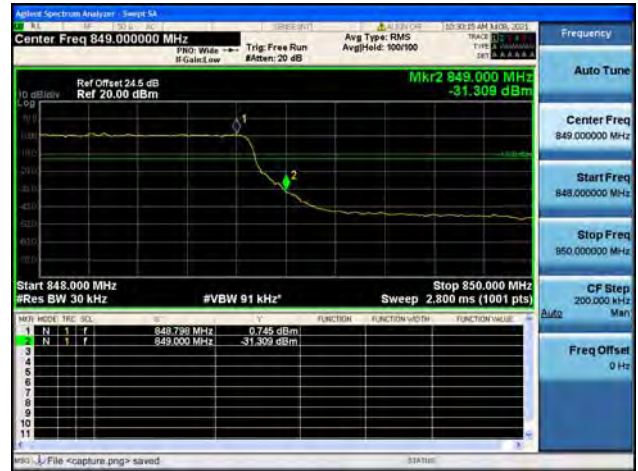
Band5 / 5MHz / Low CH / QPSK / FULL RB
