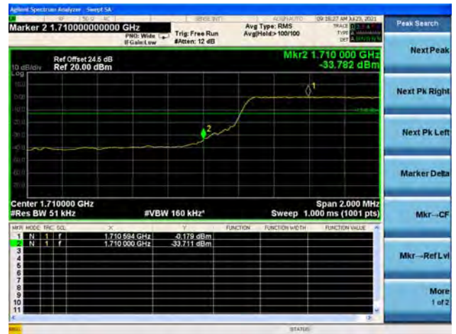
Band66 / 5MHz / High CH / QPSK / FULL RB
