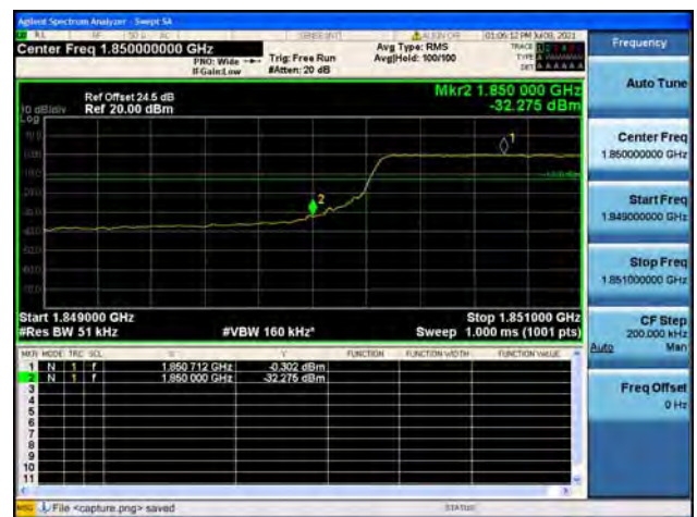
Band2 / 5MHz / High CH / QPSK / FULL RB
