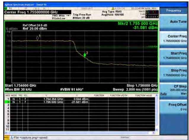
Band4 / 5MHz / Low CH / QPSK / FULL RB
