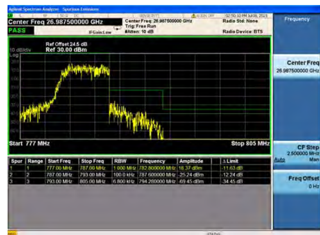
Band13 / 5MHz / High CH / QPSK / FULL RB
