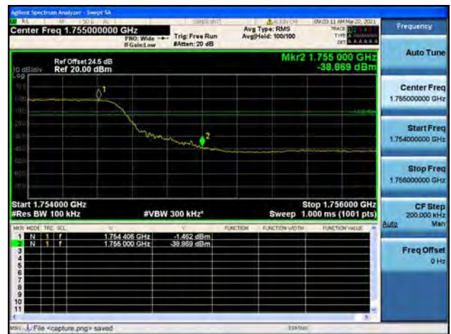
Band4 / 15MHz / Low CH / QPSK / FULL RB
