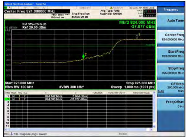
Band5 / 10MHz / High CH / QPSK / FULL RB
