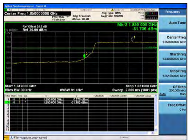
Band2 / 3MHz / Low CH / QPSK / FULL RB
