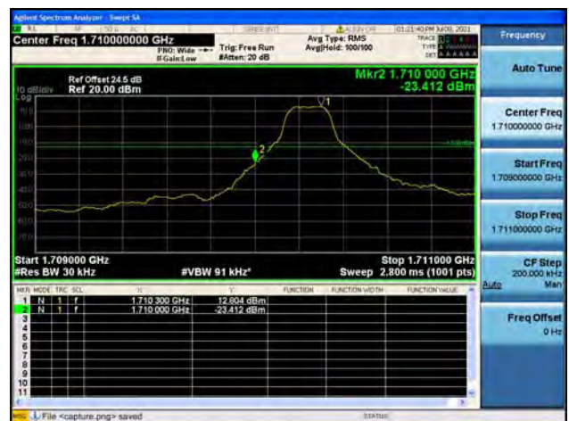
Band4 / 3MHz / Low CH / QPSK / FULL RB
