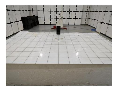
**Set-up for Radiated Spurious Emission, Above 1GHz**
