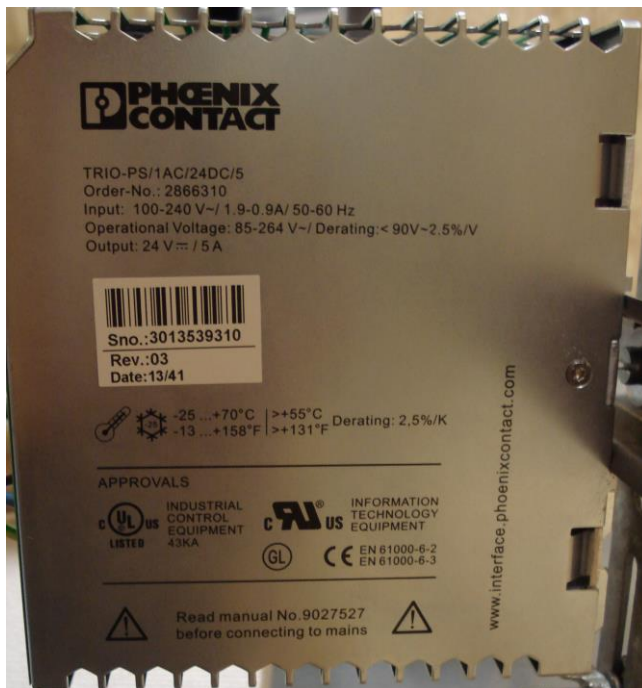
Photograph 2.3-1: Power supply TRIO-PS/1AC/24DC/5
