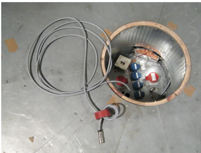
Photograph 2.3-3: Junction box with signal and supply cable and ferrite connected
