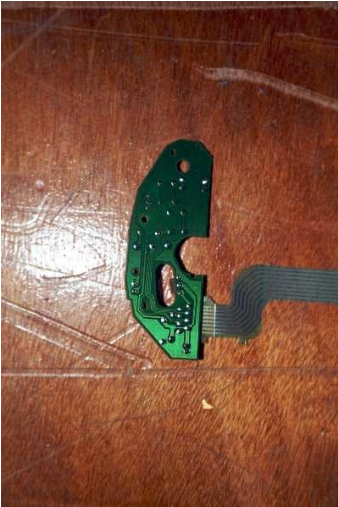
BOTTOM VIEW OF MOUSE CIRCUIT BOARD (Y-RE20)
