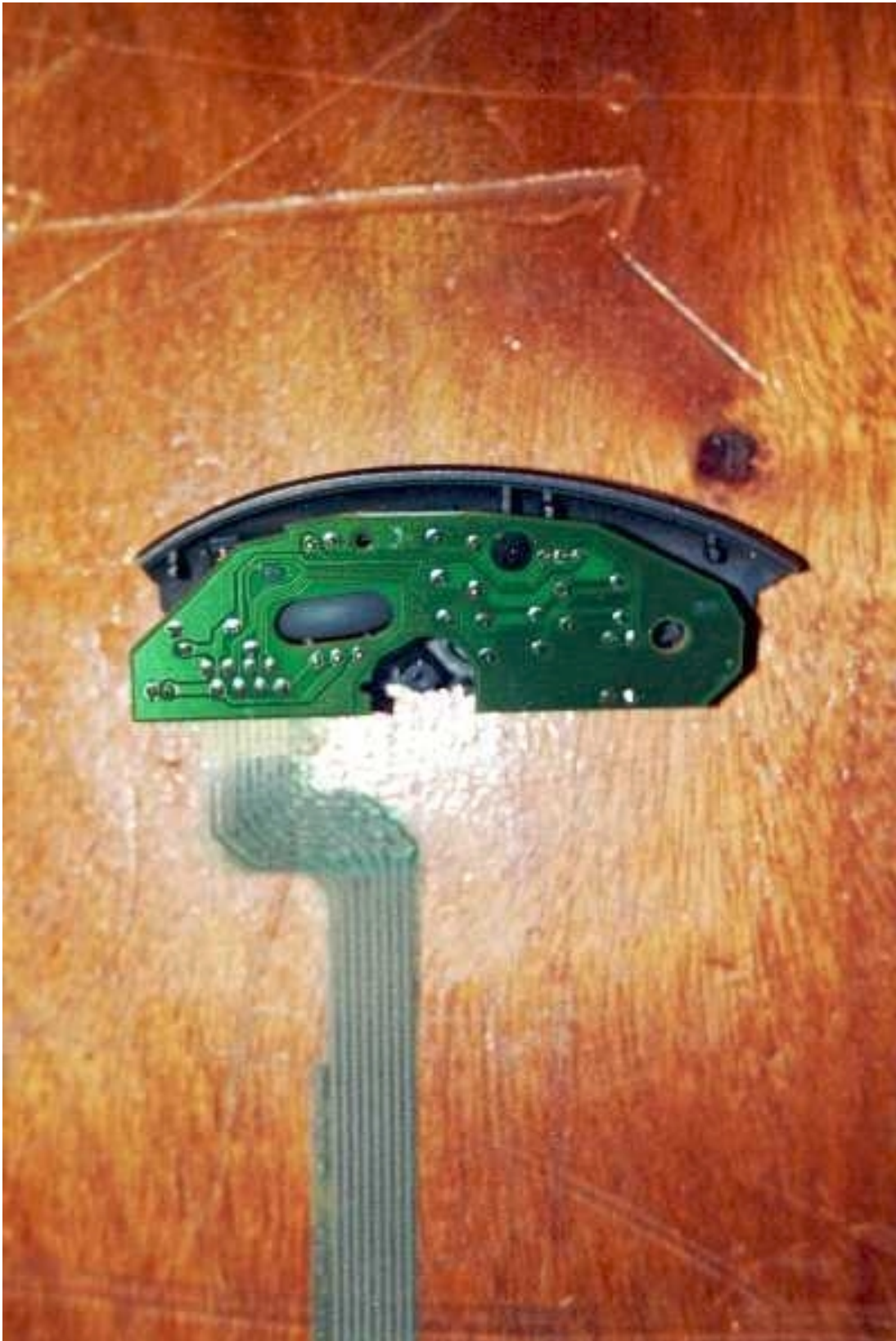
BOTTOM VIEW OF MOUSE ASSEMBLY (Y-RE20)
