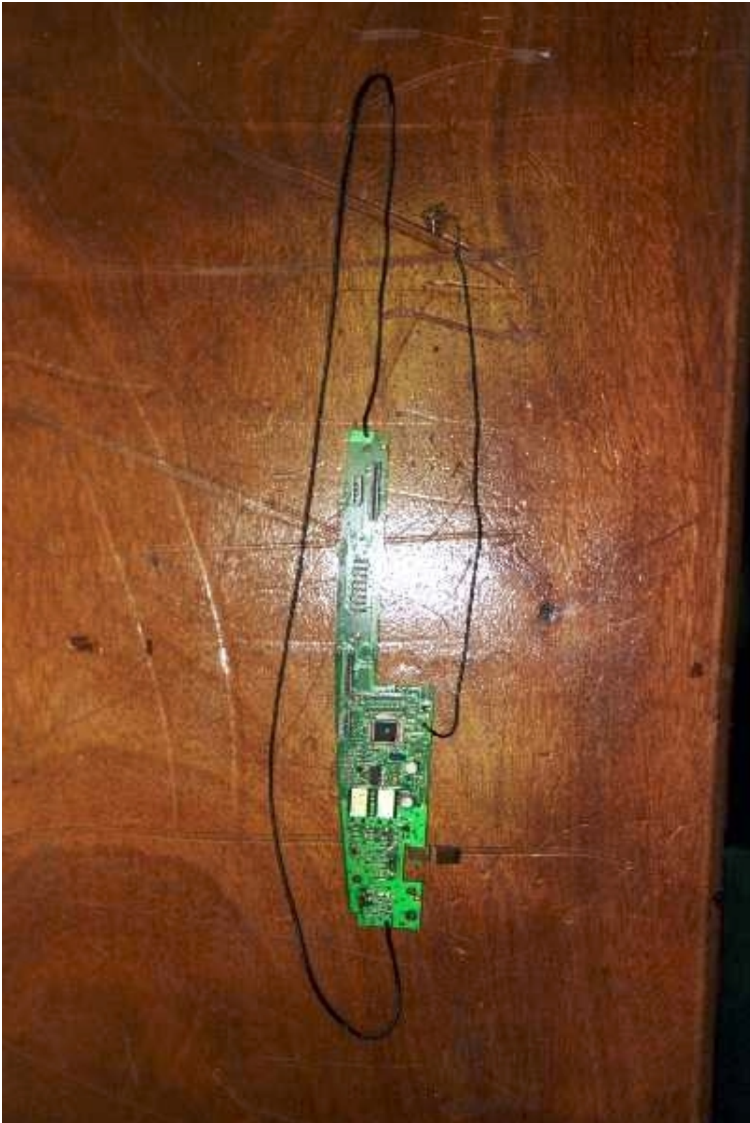
TOP VIEW OF TRANSMITTER BOARD/ANTENNA (Y-RE20)
