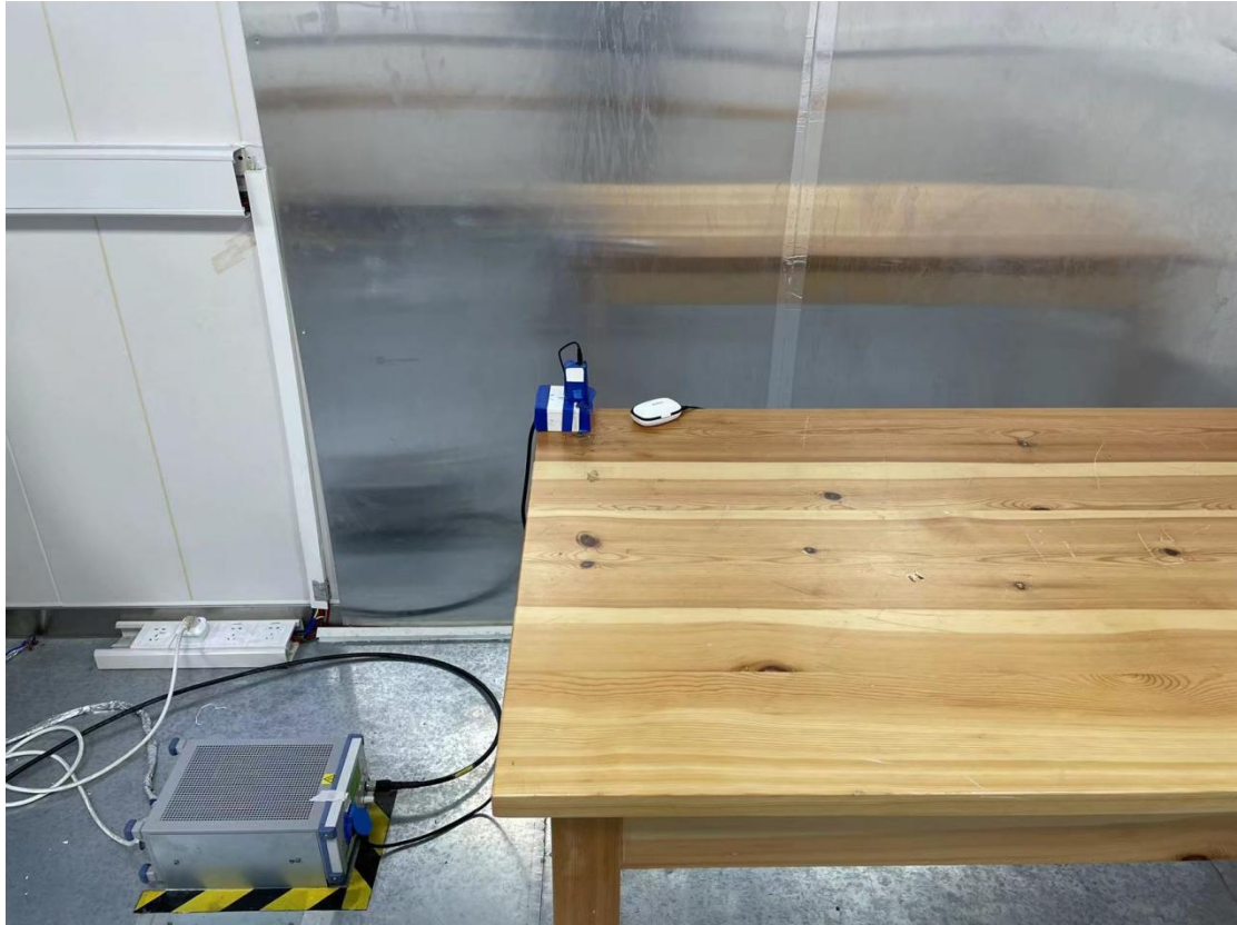
Conducted emission test setup
