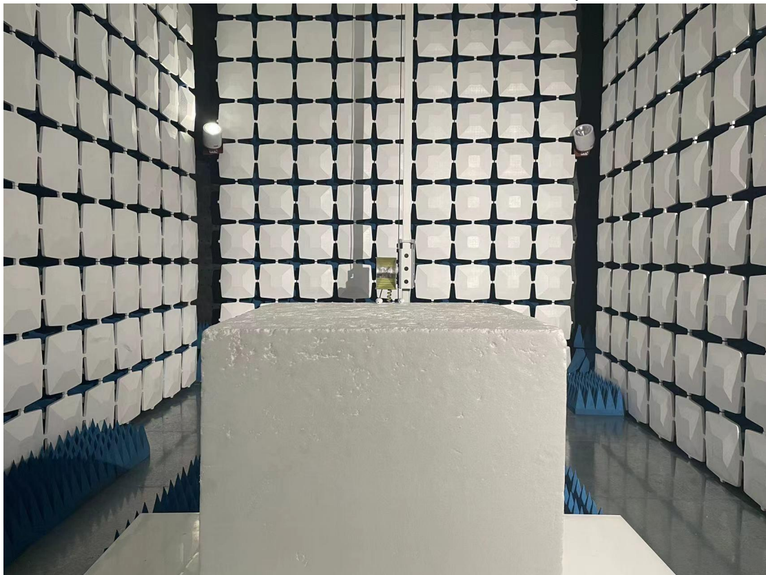
Above 1GHz for radiated emission test setup
