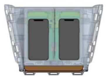
NOTE: The Wireless Phone Charger many not work if the phone case is too large or made of metal. Take the phone out of the case and place the phone on the charger in the above-mentioned cases.
