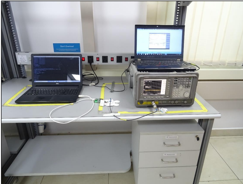
Conducted test setup
