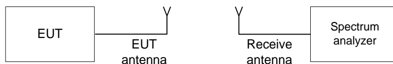
Figure 7.1.1 The 20 dB bandwidth test setup
