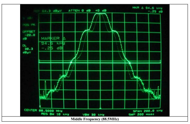
According to Section 15.31(m), only middle channel was observed.
