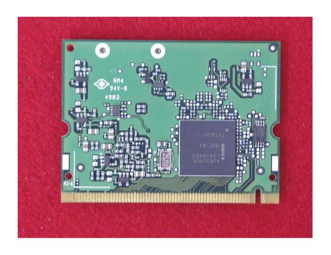
Bottom View of the WLAN Transmitter "Insulation Removed"
