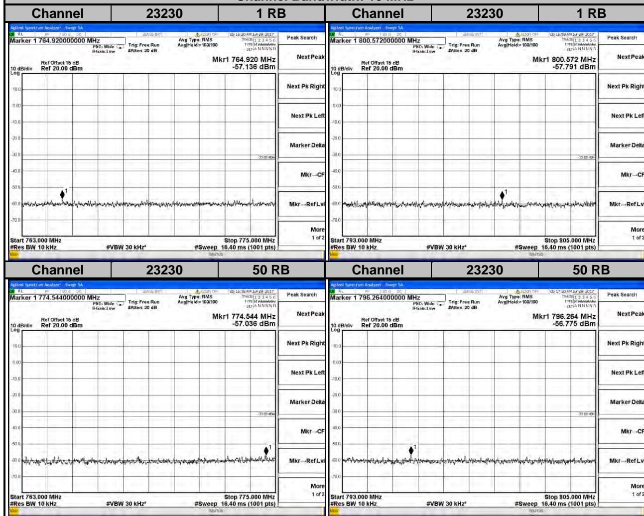
For the 763 - 775 MHz and 793 - 805 MHz band ,the FCC limit is  $65+10\log(P[\text{watt}])$  in a 6.25 kHz bandwidth . Since it was not possible to set the resolution bandwidth to 6.25 kHz with the available equipment , a bandwidth of 10 kHz was used instead to show compliance. By using a 10 kHz bandwidth on the spectrum analyzer.
