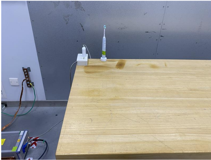
Conducted Emissions test setup photo
