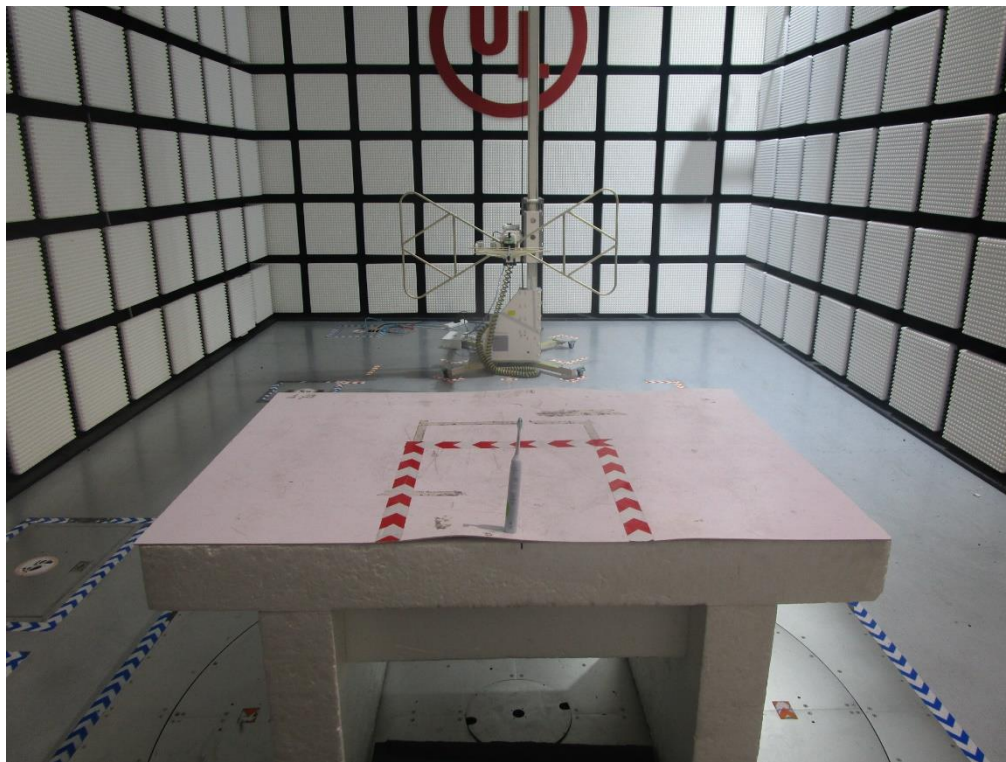
Radiated Emissions below 1 GHz test setup photo
