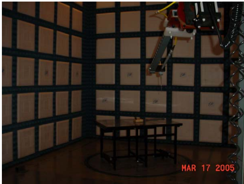
Test Set-up for Radiated Emissions Vertical Polarity
