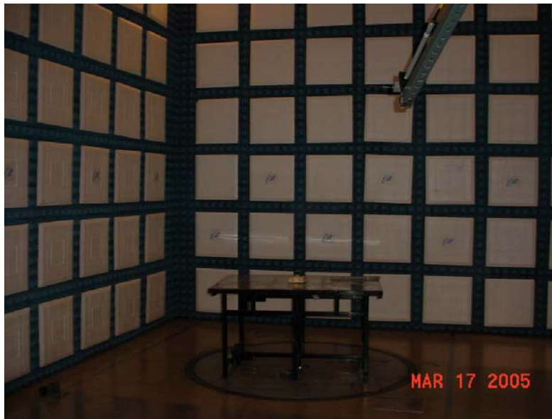
Test Set-up for Radiated Emissions Horizontal Polarity
